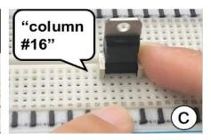
Figure 1: AccessibleCircuits system. (a) Braille text describing the value of a resistor's color stripes; (b) 3D printed add-on adaptations for potentiometer with wire slots; (c) User touching the component add-on to trigger audio feedback.
