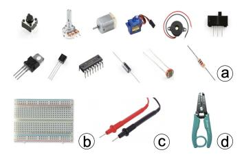
Figure 2: (a) Components include a button, potentiometer, motor, servo, buzzer, slide switch, transistor, temperature sensor, 16-pins IC, diode, photocell, resistor, (b) half-size breadboard, (c) probes, (d) and a wire stripper.
