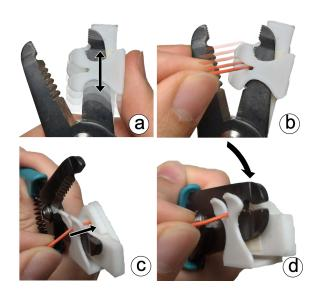
Figure 10: Illustration of the wire stripper adaptation. (a) Slidable blade slot selector. (b) V-shaped wire guide that holds a wire in the desired blade slot. (c - d) Users can move the wire and cut at a pre-set length.
