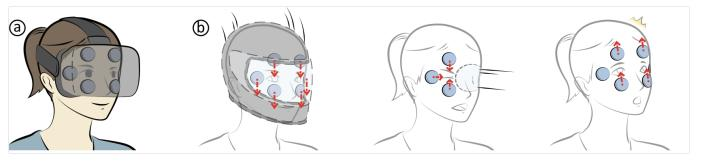
Figure 1. Masque is a prototype HMD integrating with six skin stretch modules. (a) Six shear tactors are placed on the facial interface and can generate 2-degree-of-freedom lateral skin stretches, (b) which enables various skin stretch feedback or directional cues in virtual reality.
