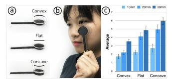
Figure 2. (a) The shear tactors we explored, including convex, flat, and concave shapes. (b) The participant generates skin stretches by the tactors. (c) User preferences regarding the shear tactors. Error bars show a standard error in all figures.
