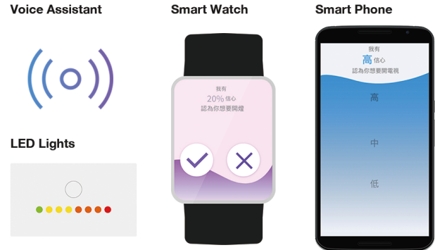
Figure 2. The four user interfaces used in this study. The message on the smartwatch reads, "I have 20% confidence that you want to turn on the lights", and the one on the smartphone says, "I have high confidence that you want to turn on the TV". The former was printed on cardboard while the later was an interactive prototype
